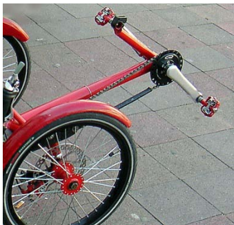
Figur 9-50: Schlumpf High Speed Drive monterad i en tadpole-trike. Observera den kompakta storleken
